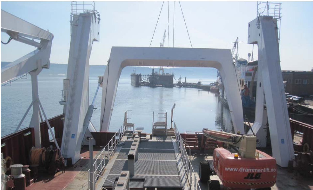
A-Frames for Cable handling incl. handling of Cable Deployment Bow
